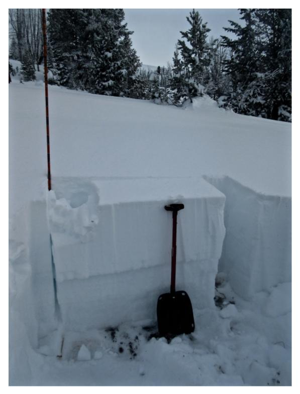
We rode into Cabin Creek behind Sage Peak (via Taylor Fork) and found 2.5' of snow. The lower half was weak, sugary and unsupportive. The upper half was a slab of recent snow that collapsed with moderate force (ECTP 11). Our sled's tracks easily broke through 2.5' of snow to the ground, a sign of poor snowpack structure. Photo: GNFAC
