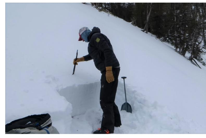
This 2-foot deep snowpit consisted of layers of crusts and facets. It was dug on a SW aspect at 9800' in Miller Drainage. Nothing broke clean in our stability tests and we are optimistic about it handling a load of new snow. Photo: GNFAC
