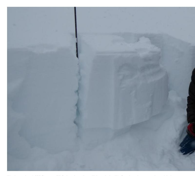
We dug a pit at 9,000 feet on a SE facing slope above Hebgen Lake. We found weak snow under a slab that broke with an ECTP26. Photo: GNFAC
