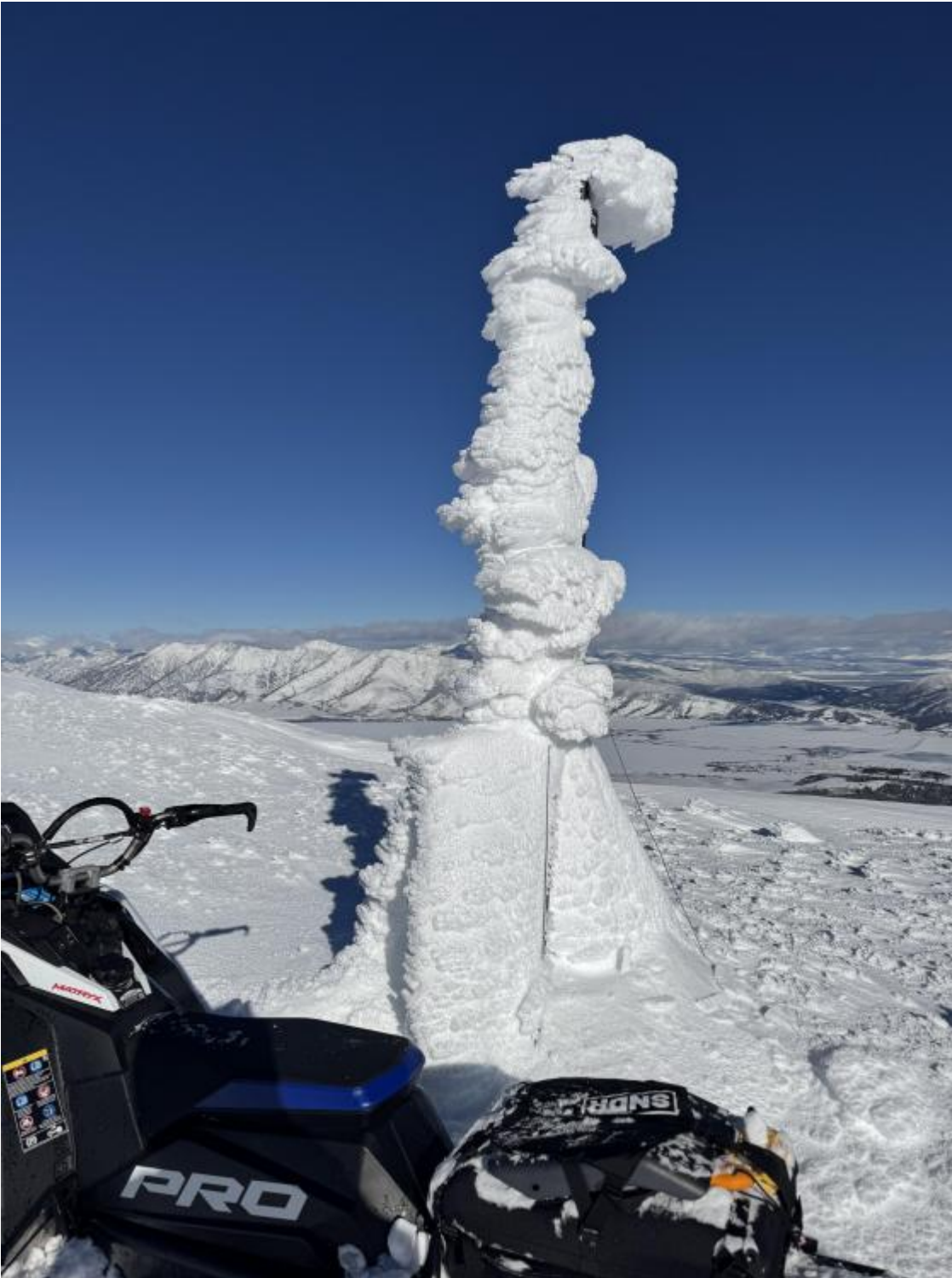
The GNFAC weather station at the top of Sawtelle provides wind, temperature and relative humidity information for forecasting (when it's not covered in a foot of rime ice. Photo: GNFAC
