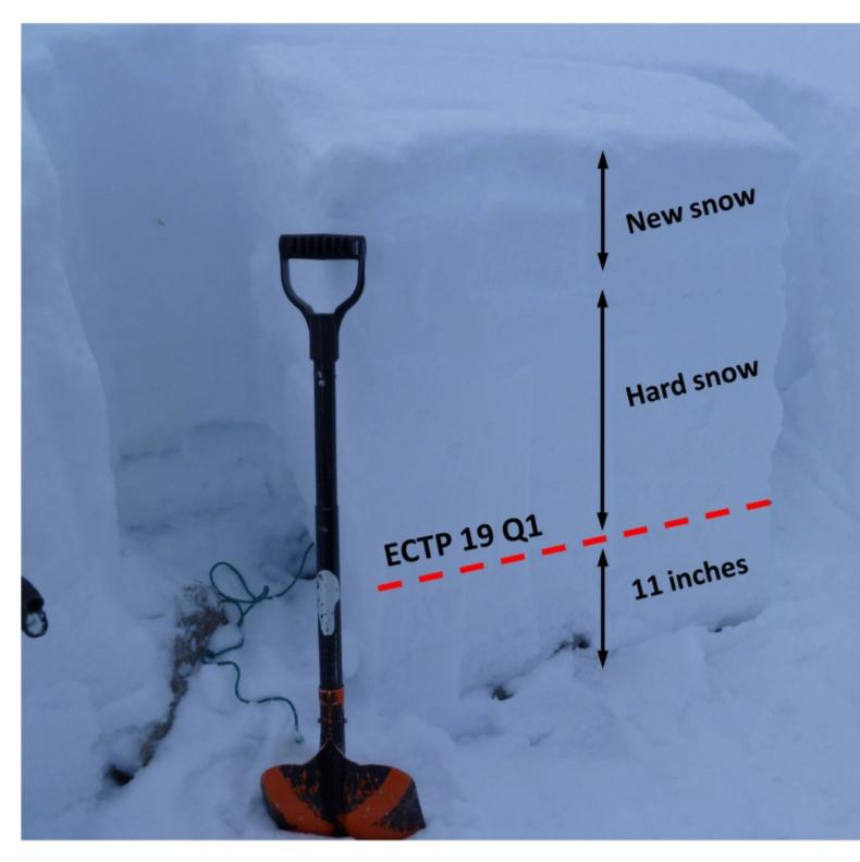
This pit was dug between Fairy and Frazier lakes in the northern Bridger Range. Faceted crystals 1-2 mm in size near the interface between October snow and November snow were found. They were obvious in the snow pit and produced stability test results that indicated their weakness and potential to produce an avalanche.
