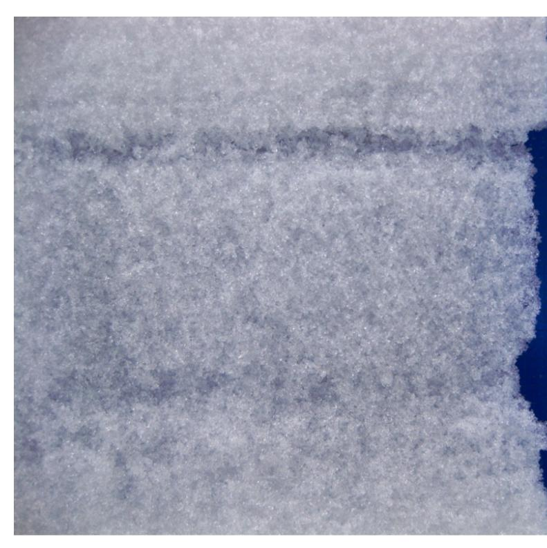
The upper stripe in the photograph is a layer of surface hoar buried 45cm off the ground. It is breaking clean in our stability tests (ECTP22 and 27). Mark found this layer in Taylor Fork on Dec 5 and had ECTP12...so it's likely gaining strength. Surface hoar is scary because it has a tendency to break far and wide, sometimes unexpectedly. Photo: GNFAC
