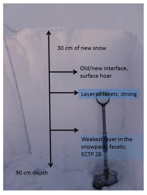
This snowpit was dug on the south side of Carrot Basin. The layer of most concern is 26cm off the ground: a layer of sugary facets. The snowpit profile is **HERE**.
