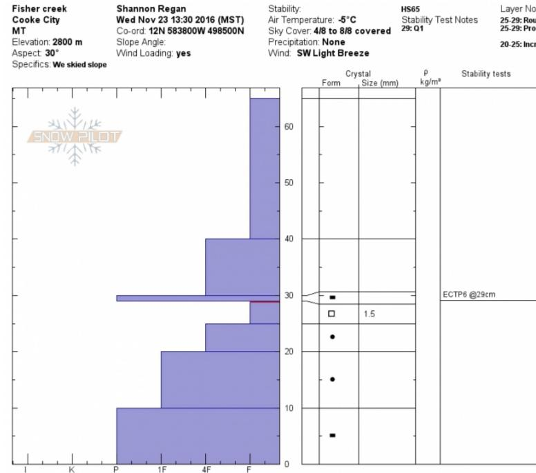
Notes: After the first ectp on the ice/faceted interface on a 17 degree slope we dug two more ect s within 50m area on approximately North facing as degree slope with propagation upon block separation, the other on a 10 degree slope with ectn 11 on the same layer.
